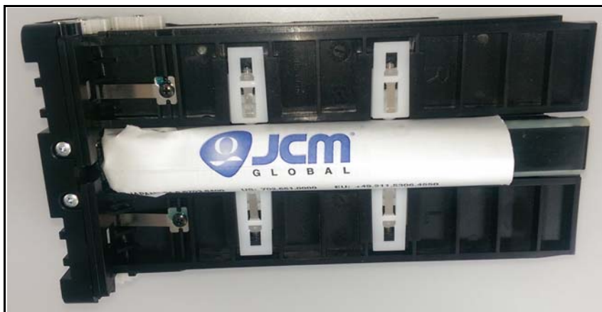
Figure 1: iVIZION Cash Box Stacker Assembly with Ticket Jam (Abnormal)
