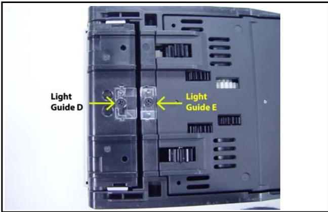
Figure 1: TR Light Guides D and E (iVIZION® Transport and Transport Cover)
